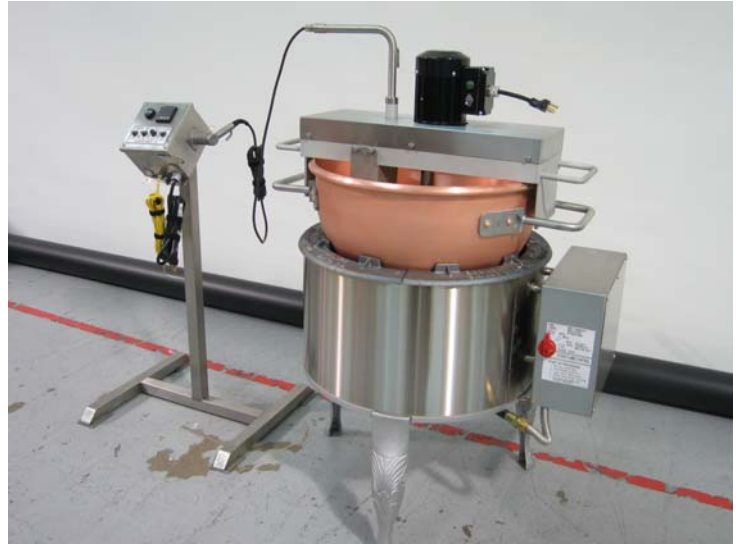
Digital Stove Controller on optional stand shown with special #20 Gas Stove equipped for external control
