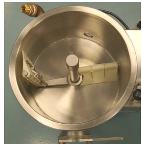
View of agitator with spring-loaded scrapers Easily removed for cleaning without tools
