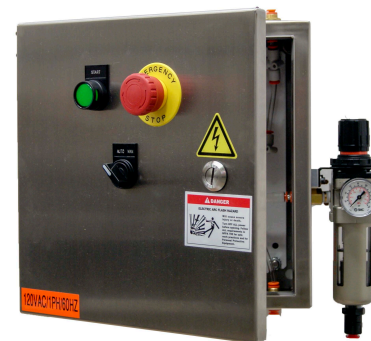
This panel features an electro-pneumatic design and provides the controls for despositor machinery. ECT provided design assistance, procured the material and fabricated the panels for an OEM.
