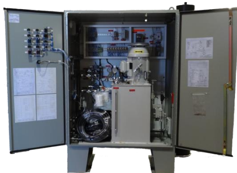
This panel is an Electro/Hydraulic control for knife gate valves in a slurry pipeline that ECT designed and fabricated.
