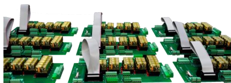
This subassembly features Relay/PLC interface boards for IDEC micro PLC's. ECT designed and fabricated this based on the customer's specification.
